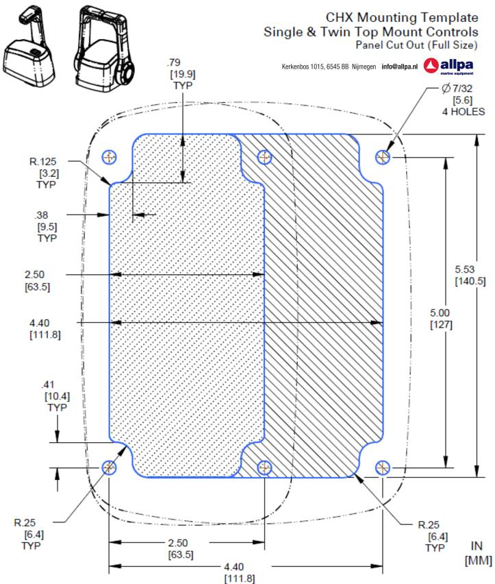
REMOVE ENTIRE HATCHED AREA WHEN MOUNTING BOTH SINGLE & TWIN CONTROLS ON TOP OF PANEL.
